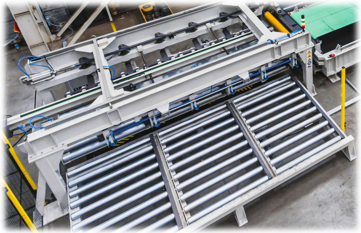
Fig. 5-8 – Automatic sheet stacking module, design example
