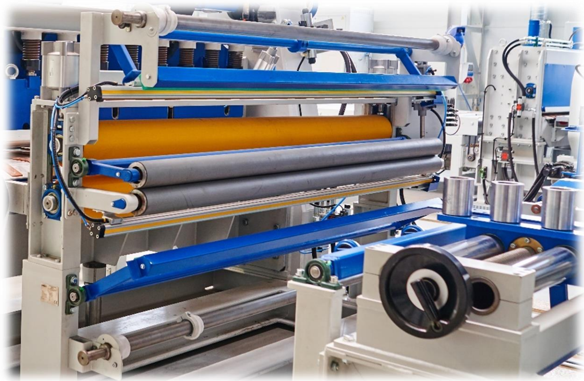
Rys. 5-5 – Double-sided folding band system
