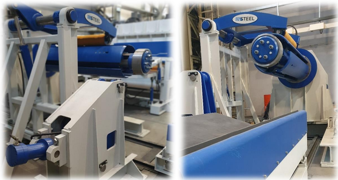
Fig. 5-1 – Strip uncoiler 7.5 t
