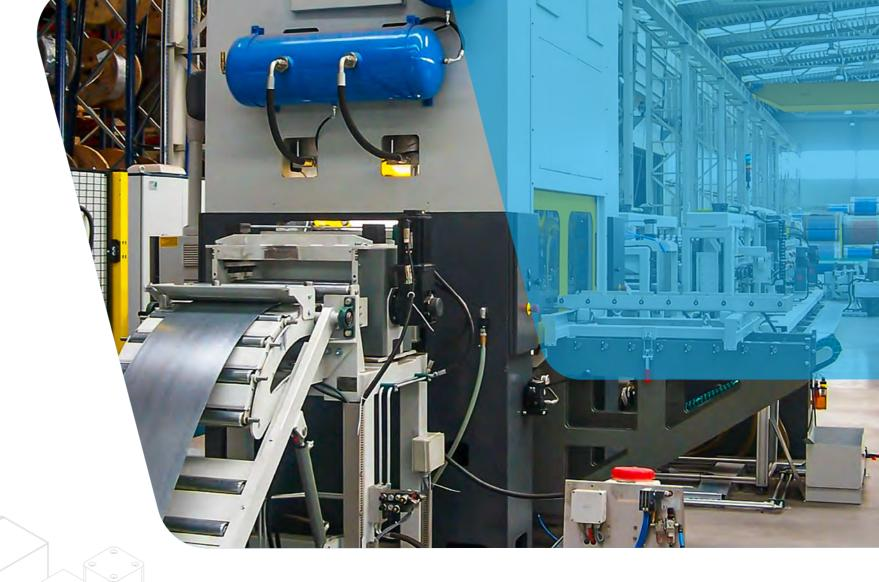
The feeder operates in two modes: a continuous cycle in line with the press speed or a single cycle.
