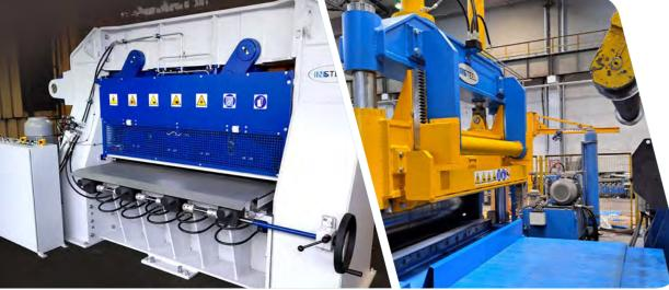
Our shears use a segmented cutting knife system with an adjustable inter-knife gap, which greatly simplifies maintenance operations.
